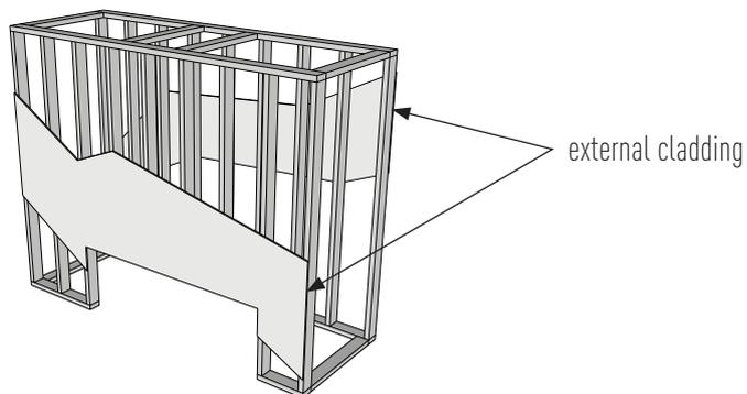
The framing structure must be clad **externally** with non combustible material and gaps sealed with a non-combustible fire proof sealant. We recommend the fireplace to be in position and flued prior to cladding.
