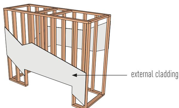
The framing structure must be clad **externally** with non combustible material and gaps sealed with a non-combustible fire proof sealant. We recommend the fireplace to be in position and flued prior to framing/cladding.
