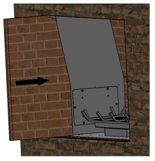
5. Insert the brick holders for each side, as shown.
