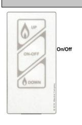
**ON:** Press and hold the **ON-OFF** button until two short beeps confirms the start sequence has begun; release button.
