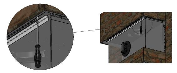
Take all the bottom bracket screws out. Then, remove the bracket.
