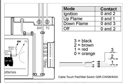
Wiring Diagram and Operation Sequence
