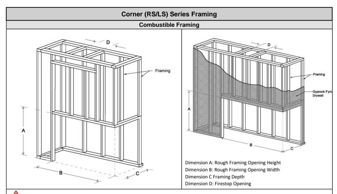
WARNING – MAINTAIN AIR FLOW CLEARANCE: Firebox top flue must have minimum 10 cm of clearance to any material achieve sufficient airflow. Failure to do so could result in improper fireplace operation, property damage, or physical injury. Review "General Clearances" section prior to framing to ensure all clearances are followed.
