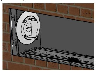
Remove the screws from each holder, and take the holders out.
