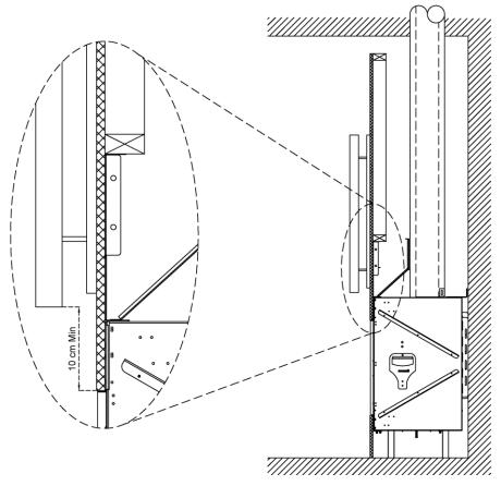
NOTE: Flue clearances must be maintained. See "General Clearances" section for details.
