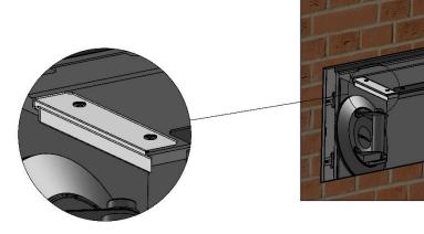
4. Remove the side panel:Lift the panel up, as shown:
