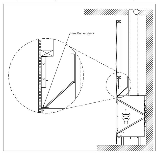
NOTE: It is acceptable if the flat stud immediately above the fireplace hangs over heat barrier flues *slightly* when using standard metal framing (as shown in diagram above).
