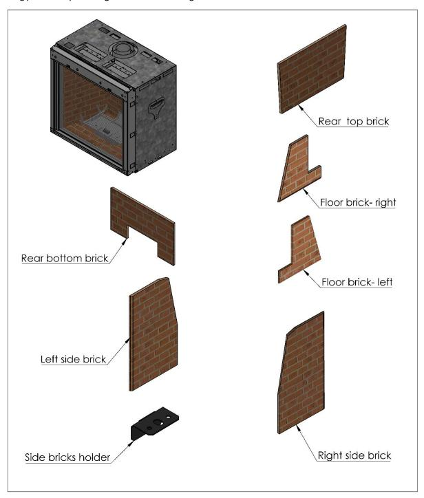
Figure 5: Components for Traditional Bricks Installation
