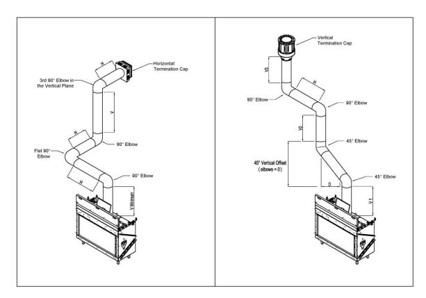
TERMINATION CAP NOTE: Low Profile Vertical Termination Cap and Sconce Horizontal Termination Cap can negatively impact flame appearance and are not recommended for use with the fireplace.
