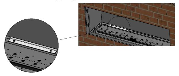
If the screws on the starter collar are type (M10), remove them as shown in the figure below. Do NOT remove Phillips screws from the starter collar.
