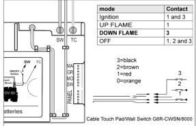
Figure 1: Wiring diagram and the operation sequence
