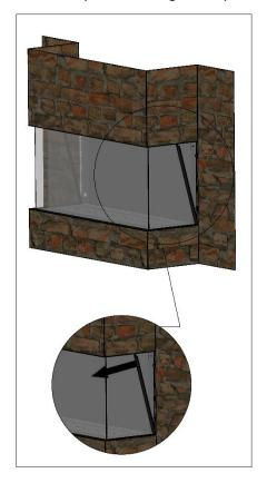
Continue pulling the side trim until it is disconnected from the bottom magnet.
