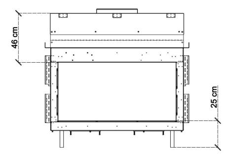
NOTE: An air intake is necessary to incorporate into the platform depending on the design. See "Air Intake for a Platform" for details.
