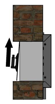
Pull the suction cup from the bottom until the glass clears the frame.
