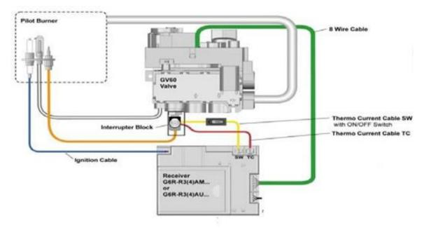
Figure 12: Valve/Receiver Wires and Interrupter Block
