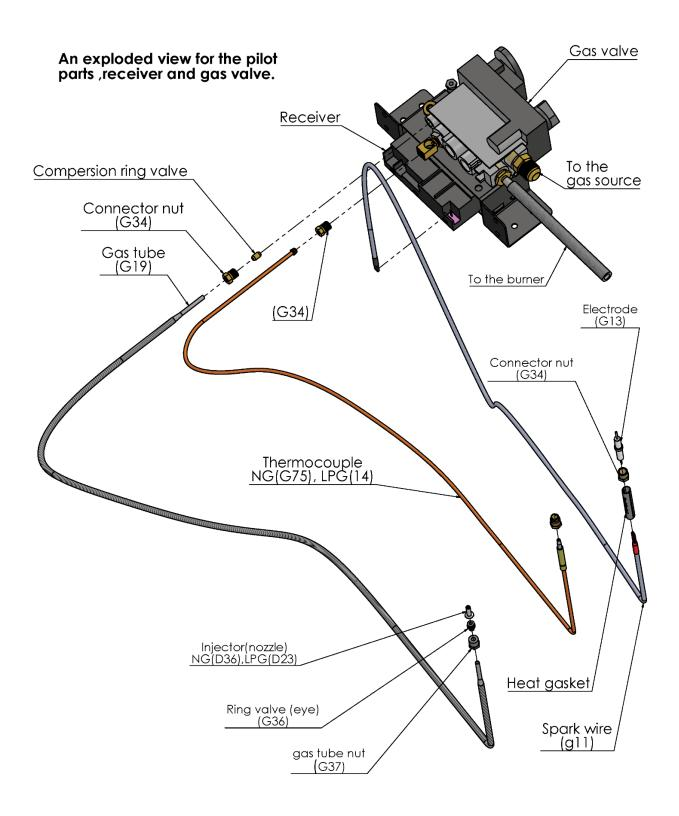
3d. Pull the wire to dissconnect it from the receiver, (as shown in figure (3)).
