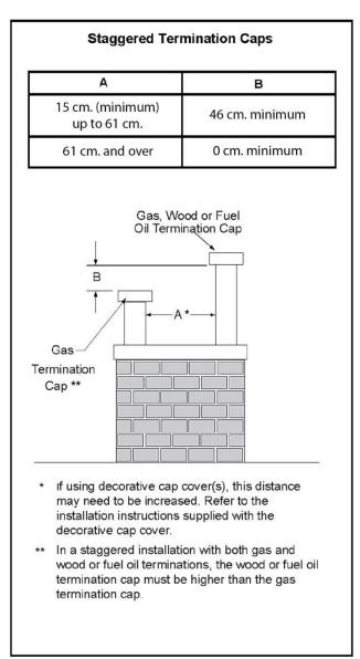
NOTE: This chart does <u>not</u> apply to a chimney shroud application. See the "Chimney Shroud" section on the following pages for more information.
