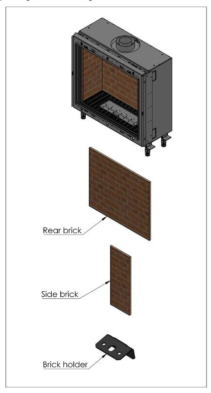
Figure 4: Components for Front Bricks Installation
