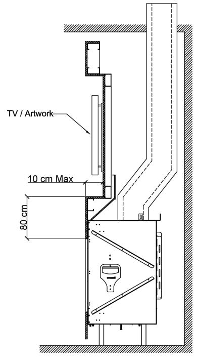
NOTE: Flue clearances must be maintained. See "General Clearances" section for details.
