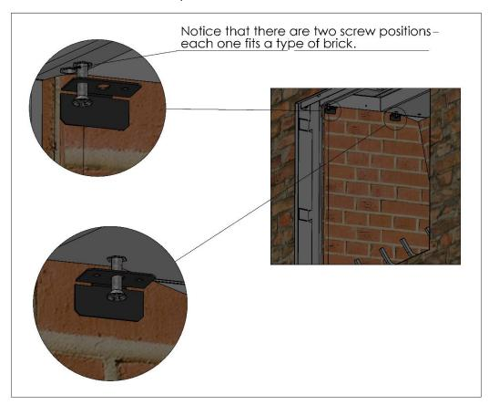
NOTE: The side bricks hold the rear bricks.
