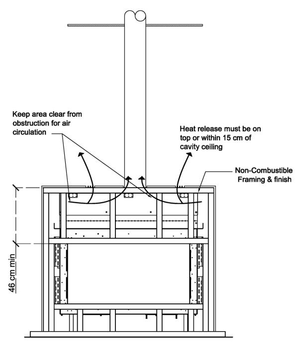
**Minimum Cavity Ceiling Clearance Diagram**
