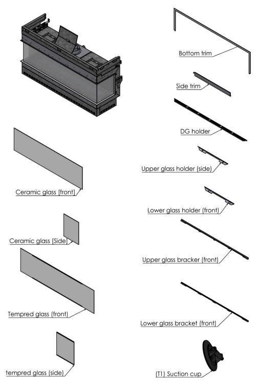
Figure 2: Double Glass Heat Barrier: Parts
