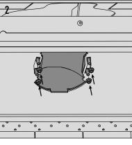
**Caution**: Attach the nozzle to the fireplace using self-tapping screws. Three holes are fitted for this purpose in the cast iron flange [diagram 5].
