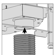
The outside air supply for combustion can be done on the right or on the left of the air box.
